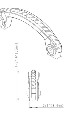
ACCESSORY: SCREW:8-32XI" 2PCS BREAK AWAY SCREW:8-32x45 2PCS ALL SCREW MATERIAL:STEEL-SAE1006
