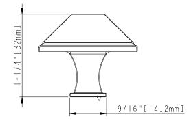
ACCESSORY: SCREW:8-32XI-1/8" IPCS BREAK AWAY SCREW:8-32x45 IPCS ALL SCREW MATERIAL:STEEL-SAE1006
