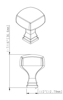
ACCESSORY: SCREW:8-32XI" IPCS BREAK AWAY SCREW:8-32x45 IPCS ALL SCREW MATERIAL:STEEL-SAE1006
